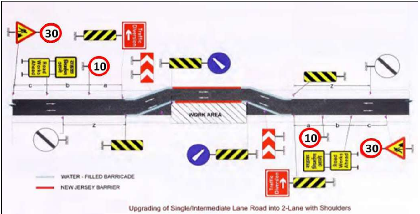
Figure 3-1: Typical Traffic Management & Work Zone Safety Arrangements
