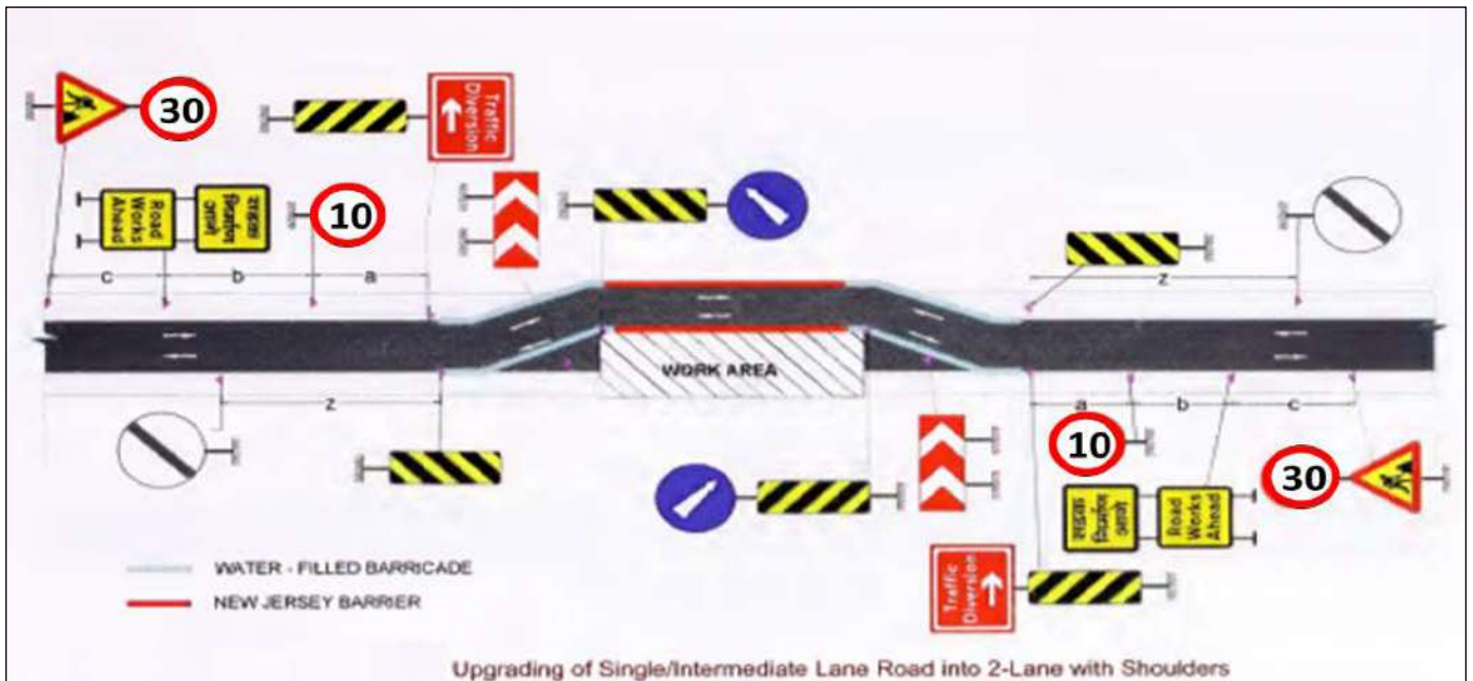
Figure 7-15: Typical Traffic Management & Work Zone Safety Arrangements
